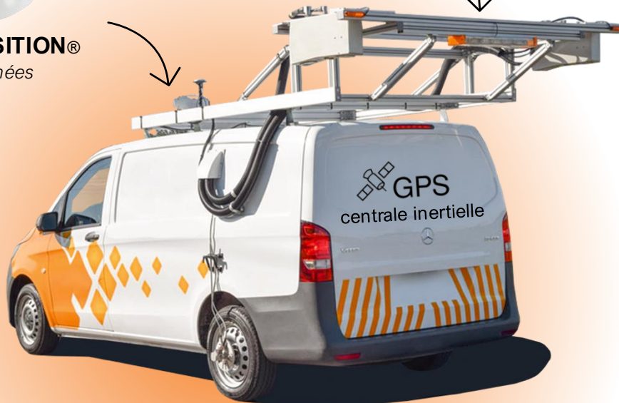
VIAPIX LCMS® Laser Crack Measurement System
